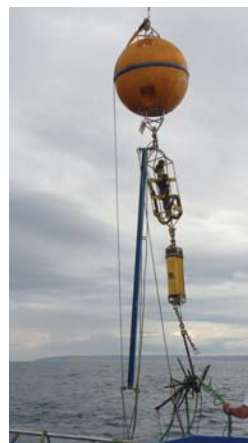
Figure 2: Bottom of the reference station after being recovered by the innovative rig.
